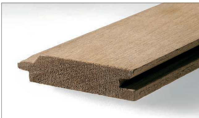
Figure 19. An example of cladding panels (ayous).
