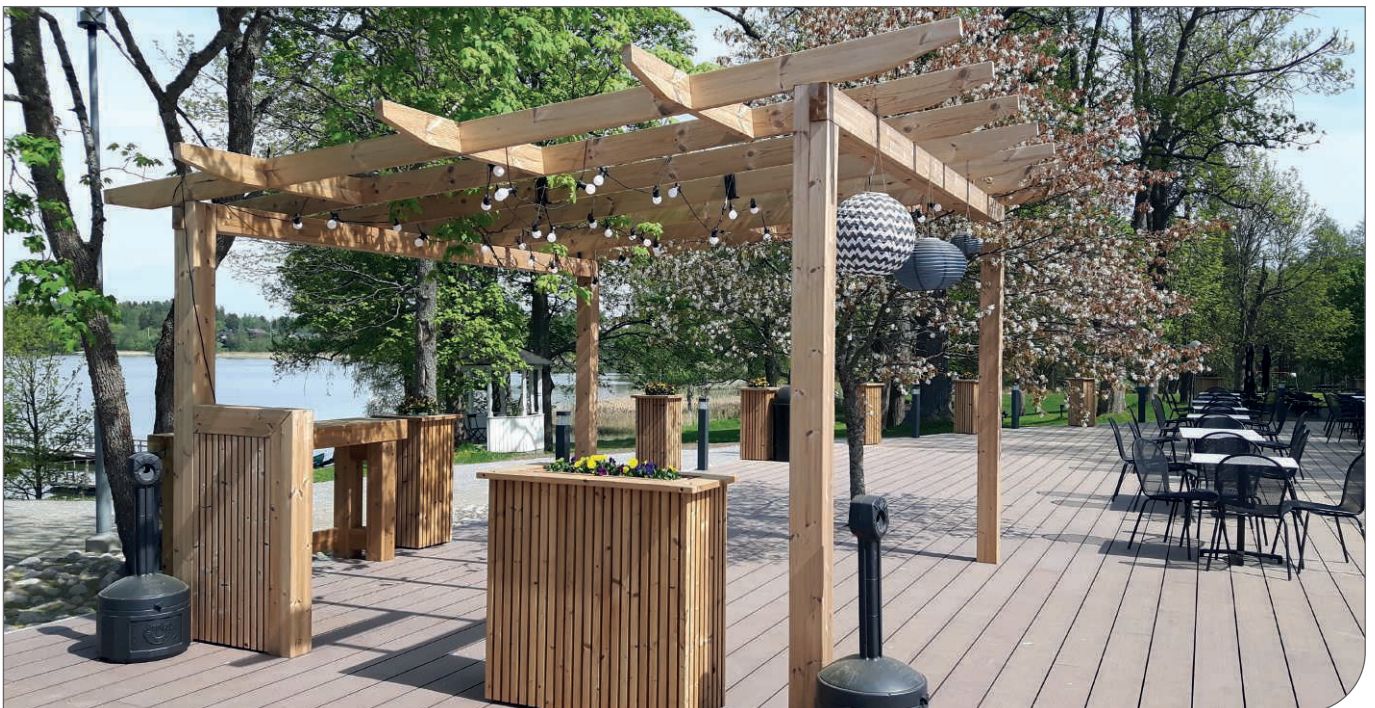
Figure 33. ThermoWood® glue beams in pergola structure
