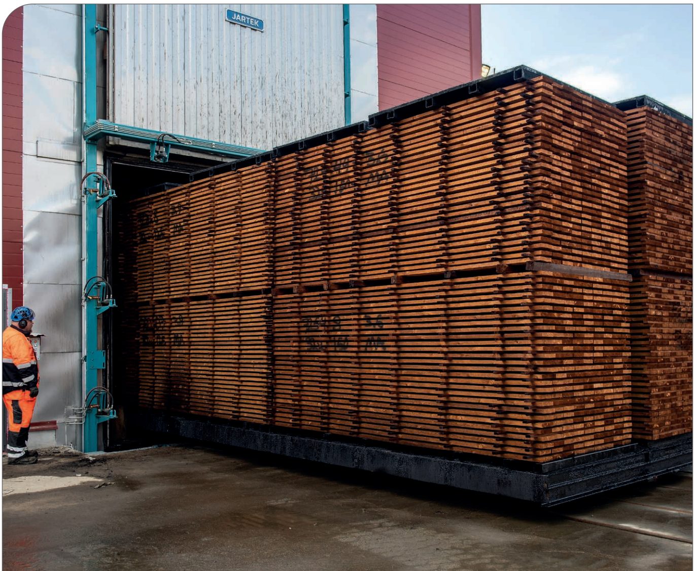
Figure 4. ThermoWood® being manufactured in process kiln.
